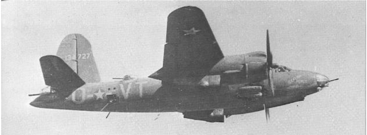
Ticklish Percy 41-34727 VT-O, a 453 rd Squadron plane in flight. The “VT” on the plane’s fuselage indicates that this plane is from the 453 rd squadron. The “O” is the individual plane’s marking, and together they make the radio call sign. This photo was taken before the distinctive white stripes were installed on the 323 rd Group’s vertical stabilizer (tail fin) - the white stripe was the identifier of the 323 rd Group ( USAAF/Freeman 58 ). This aircraft was piloted first by Lt. Clifford Ghodes and then by Lt. Frederick Mingus.
